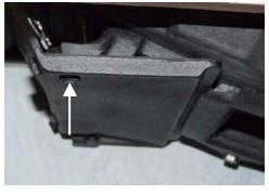
3. Using a 1/2" socket remove the two bolts that hold the bypass frame to the top of the firebox. Make sure that the gasket is also removed from under the bypass cover.
