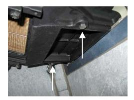
4. Install the new bypass frame using (2) 5/16"x 1" bolts. Apply anti seize compound to the bolt threads.
