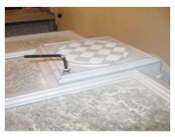
6. It will be helpful to disconnect the lift guide from the bypass cover for better access to the gasket channel. Use a ½" wrench to loosen the bolts. Prop the bypass door open. Dry fit the gasket in the channel and trim to fit if necessary. Place gasket glue into the channel. The break in the gasket should go in the center of the long length closest to the front of the stove. Re-connect the lift guide to the bypass cover.
