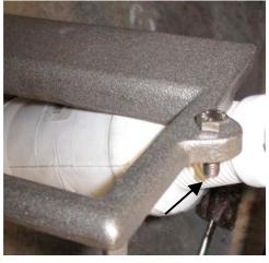
5. Replace the bypass frame gasket from the top side of the stove. The top lid of the Fireview can be removed for easy access. Keystone and Palladian owners will need to remove the cover plate with the 5/32" allen wrench to access the top area of the stove.
