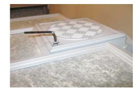
9. Replace the combustor scoop and diffuser. Place the far end of the scoop onto the support at the top of the firebox. Angle the back edge of the scoop into the lip of the bypass frame. Using (1) 5/16"x3/4" bolt fasten the scoop to the support closest to the loading door.
