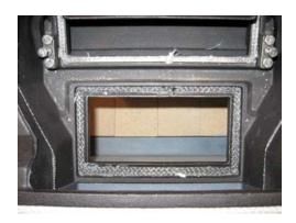
7. Check the tension on the bypass door. Slide a small piece of paper under the bypass door, close it, and pull the paper out. There should be enough resistance to curl the paper. To increase pressure on the bypass door, loosen the top nut on the U-bolt, and then turn the bottom nut counter clockwise. To decrease pressure on the bypass turn the bottom nut clockwise and do the same to the top nut. Make small adjustments until the proper seal is reached.
